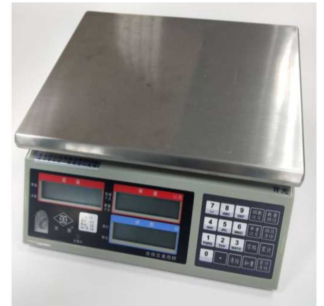
Balance for Ballast Balance capable of weighing up to 2.0 +/-0.1 kg
