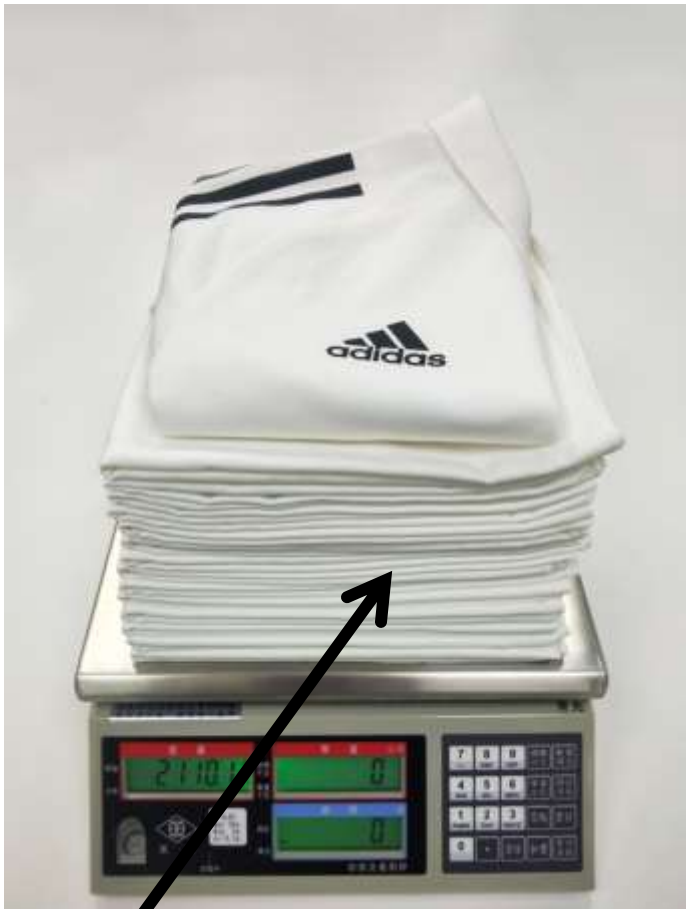
50/50 Polyester/Cotton bleached mercerized plain weave. (AATCC Ballast Type 3).
