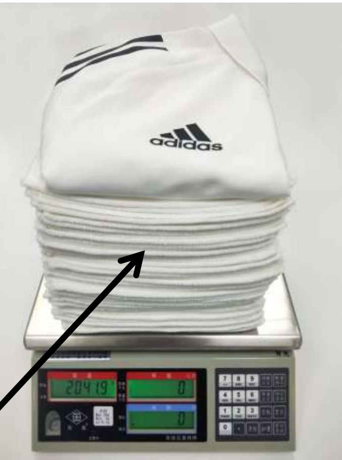
Makeweights Compliant with ISO 6330 2012 (4 layer 100% Polyester)
